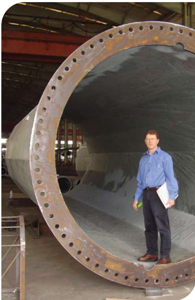
A section of one of the massive 50 metre high poles being installed in Highbrook.
